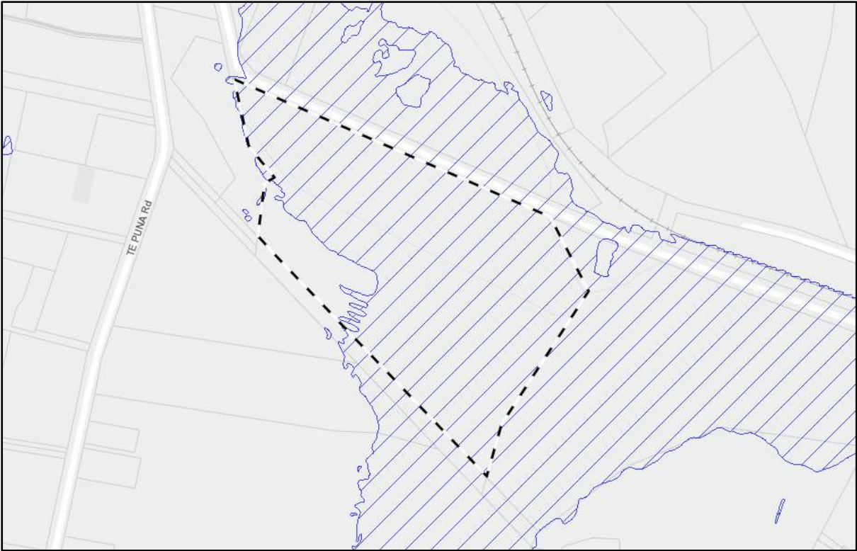
Figure 7: Extreme rainfall modelled flooding, 1:100 year climate-change adjusted event. Flood level is 3.67m RL.
