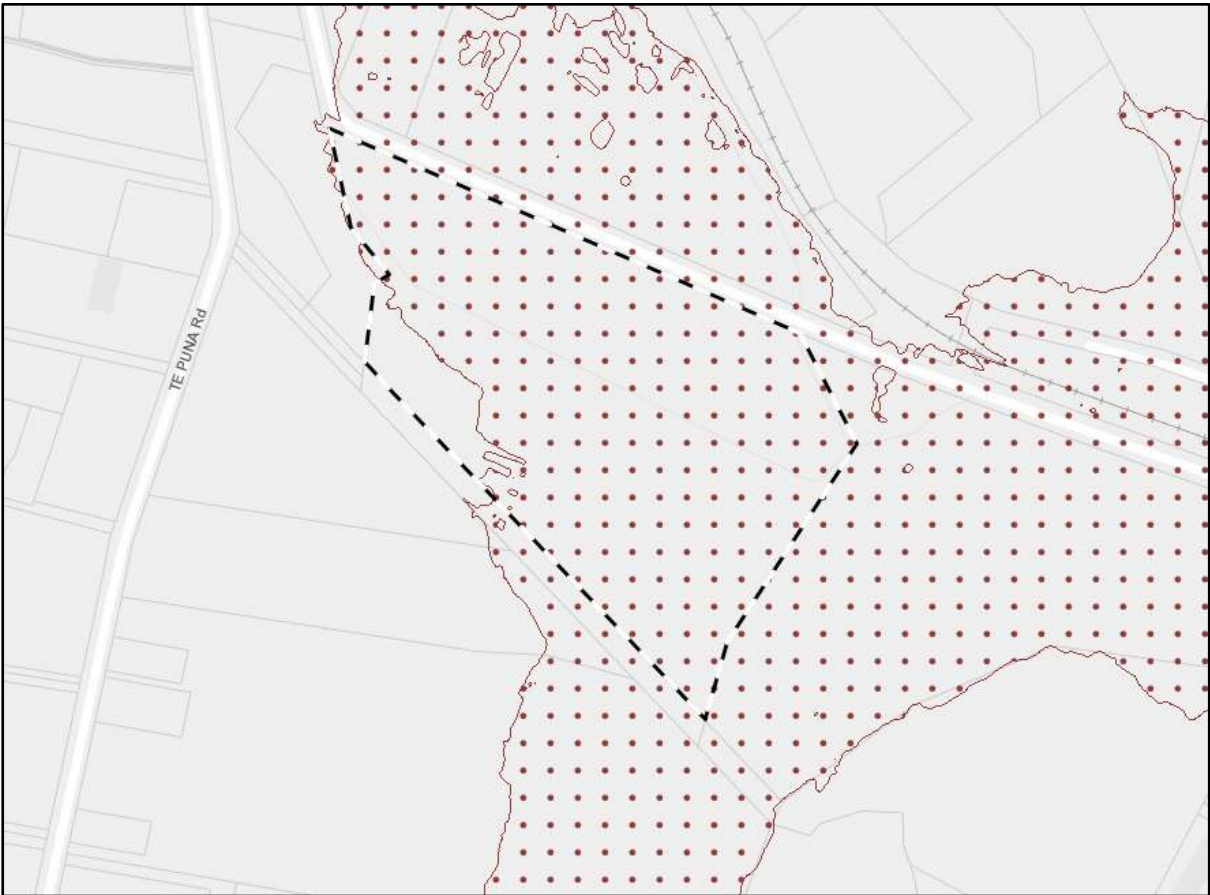
Figure 8: Coastal inundation/storm surge modelled flooding, 1:100 year climate-change adjusted event. Flood level is 3.8m RL.
